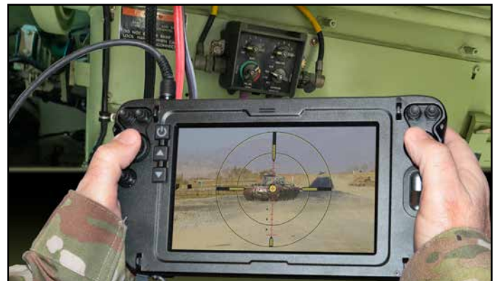
RFO enables remote operation of the turret while protected inside the vehicle.
