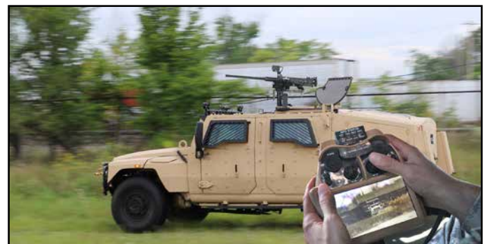
RFO enables remote operation of the turret while protected inside the vehicle.
