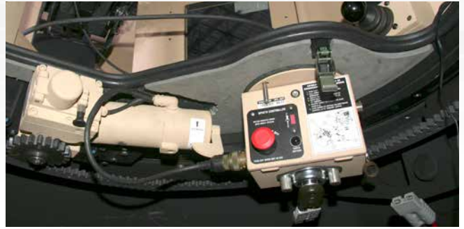
CS3249-1 (shown) TCS Motor Control and Drive Assembly
