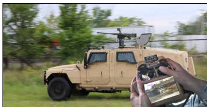
RFO enables remote operation of the turret while protected inside the vehicle.
