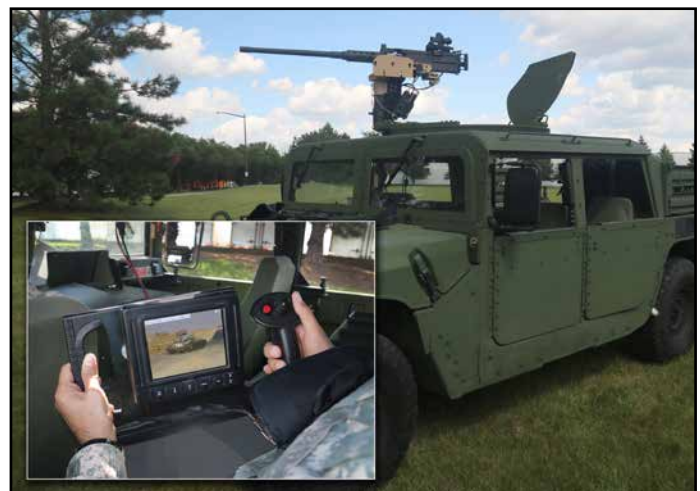
RFO enables remote operation of the turret while protected inside the vehicle
