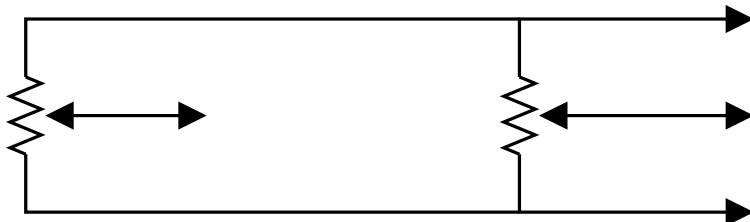
Figure 9 Maximum/Minimum Application Wiring
