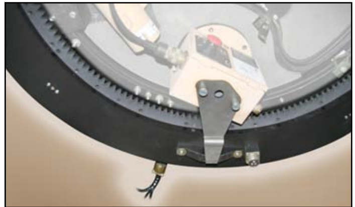
CS5400 slip ring integrated with ITDS turret controller and M1114 hatch/bearing assembly.
